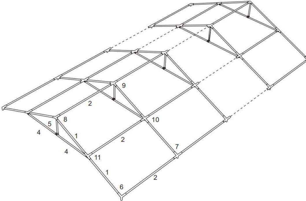
**Step 3.** Lift one side of the tent frame and attach the legs (3). Place the roof (26) onto the frame and use the bungees (22) to fasten it. Be sure not to put too much tension on the bungees in order not to make attaching the other side more difficult.
